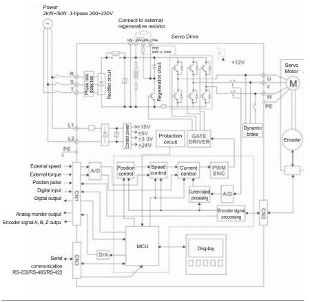
Figure 3.6 Basic Wiring Schematic of 2kW ~ 3kW models
