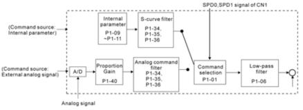
The command source is selected according to the state of SPD0, SPD1 and parameter P1-01 (S or Sz).
