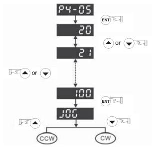
Note: JOG operation is effective only when Servo On (when the servo drive is enabled).
