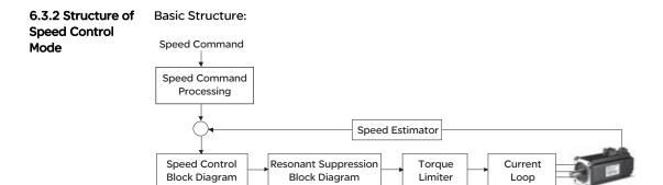
In the figure above, the speed command processing is used to select the command source of speed control according to chapter 6.3.1, including proportional gain (P1-40) and S-curve filter smoothing strategy of speed control. The speed control block diagram is used to manage the gain parameters of the servo drive and calculate the current input provided to motor instantaneously. The resonance suppression block diagram is used to suppress the resonance of mechanical system.
