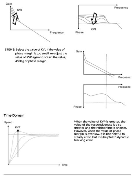
STEP 2: Fix the value of KVP and adjust the value of KVI.
