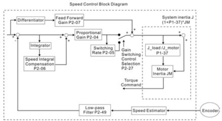
There are two turning modes of gain adjustment: Manual and Auto modes. The gain of Lexium 23 series servo drives can be adjusted by using any one of three tuning modes.
