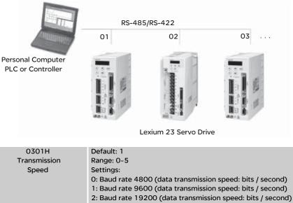
3: Baud rate 38400 (data transmission speed: bits / second) 4: Baud rate 57600 (data transmission speed: bits / second) 5: Baud rate 115200 (data transmission speed: bits / second)
