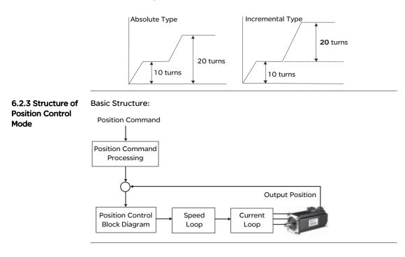
In order to pursue the goal of perfection in position control, the pulse signal should be modified through position command processing and the structure is shown as the figure below:
