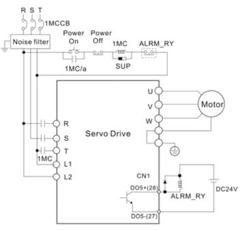
Figure 3.4 Three-Phase Power Supply Connection (for 2kW and above models)
