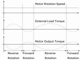
External load torque in reverse direction: TL x Wr TL : External load torque For the safety, we strongly recommend the users should select the proper resistance value according to the load.
