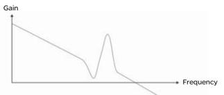
When the low-pass filter (parameter P2-25) is adjusted from 0 to high value, the value of Low-pass frequency (BW) will become smaller (see the figure below). The resonant condition is improved and the frequency response and phase margin will also decrease.
