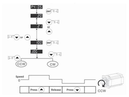
In the example below, the JOG speed is adjusted from 20r/min (Default setting) to 100r/min.
