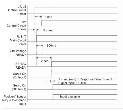
The timing charts of control circuit power and main circuit power:
