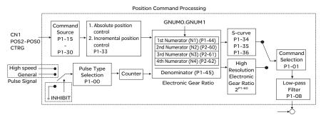
Using parameter can select Pr mode and Pt mode. Electronic gear ratio can be set in both two modes to set proper position revolution. Lexium 23 series servo drives also provide S-curve and lowpass filter, which are used whenever the motor and load need to be operated more smoothly. As for the information of electronic gear ratio, S-curve and low-pass filter, please refer to the following sections 6.2.4, 6.2.5 and 6.2.6.
