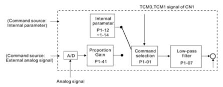
The command source is selected according to the state of TCM0, TCM1 and parameter P1-O1 (T or Tz).
