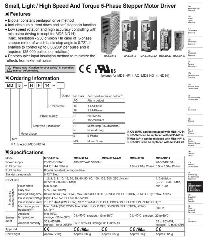
%1: When using over 30VDC, it should be mounted at ventilated place due to increasing heat.
