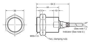
Note 1. 4-dia. vinyl-insulated round cable with 3 conductors (conductor cross section: 0.3 mm<sup>2</sup>; insulator diameter: 1.3 mm); standard length: 2 m
