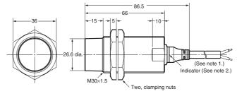
Note 1. 4-dia. vinyl-insulated round cable with 3 conductors (conductor cross section: 0.3 mm²; insulator diameter: 1.3 mm); standard length: 2 m 2. Operation indicator (yellow)
