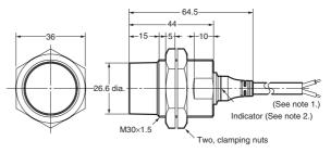
Note 1. 4-dia. vinyl-insulated round cable with 3 conductors (conductor cross section: 0.3 mm²; insulator diameter: 1.3 mm); standard length: 2 m 2. Operation indicator (yellow)
